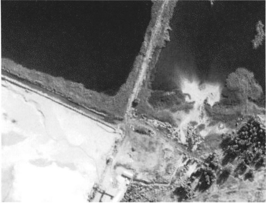
Fig. 4. Seepage of tailings into a public watercourse as seen on Ikonos imagery.
