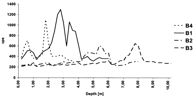
Fig. 4. Measurement of gamma-radiation along sediments of exploration drillings B1 - B4 with help of a portable differential-spectrometer.
